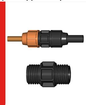
DN 15 (1/2") copper fits into 20mm Plasson compression end. Discard black 20mm Plasson nut, discard the white split ring, slide rubber liner into fitting body, position cone and SS ring inside copper coloured nut as shown in picture above. Reassemble to the Plasson body.
