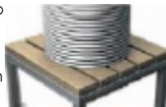
The platform must be in contact with greater than 95% of the area of the base of the tank with gaps no greater than 5mm between supports.
