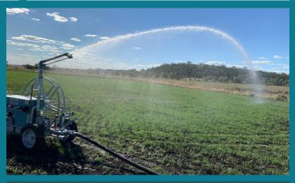
Working Pressure: 50 - 85 psi Water Flow: 400 - 900 l/min Effective Spray Width: 60 - 90 m
