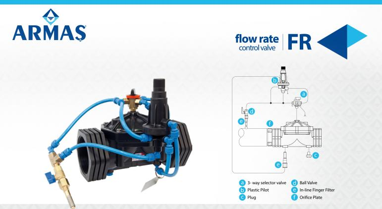
**Armaş "FR"** model flow rate control valve is designed to limit desired flow rate. The orifice on main valve upstream creates pressure difference and 3/way differential pressure set pilot mounted in control chamber of valve senses this pressure difference and ensures that main valve opens in desired flow rate. Valve thereby limits desired flow rate automatically and keeps it fixed. It eliminates over flow by preventing excessive flow during reverse washing in filtration systems.
