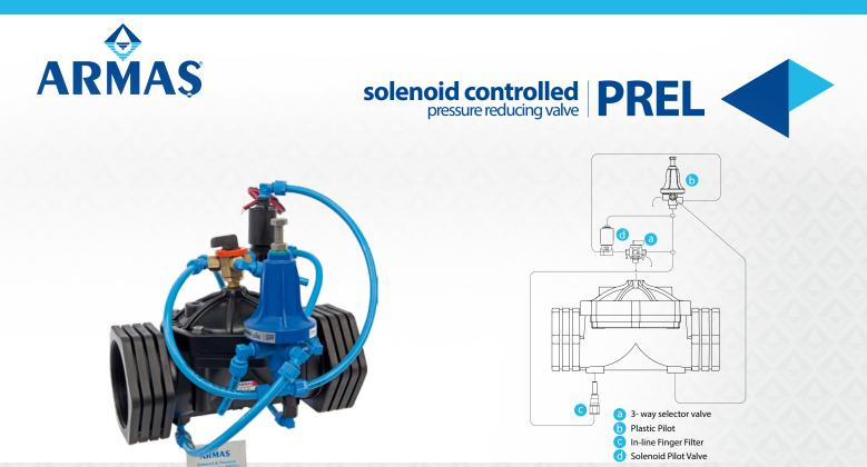
**Armaş "PREL"** model pressure reducing valve is the hydraulic control valve which reduces high upstream pressure value into desired lower pressure value. Control of main valve is achieved by means of built-in solenoid pilot valves. Electric signal for solenoid pilot valves is ensured by means of a control device, time relay, main switch and PLC control units etc. Automated control may be easily ensured by this way in application systems.
