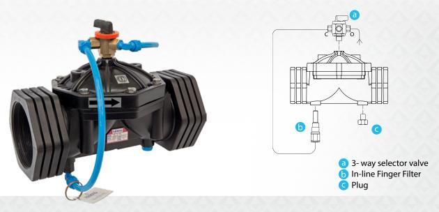
**Armaş "M"** model valve is the hydraulic control valve operated by line pressure and designed to ensure opening/closing process by means of a 3-way selector valve. Minimum opening pressure of valve is 0.7 bar. Thanks to its flexible diaphragm, it makes easy and fast control process in high pressure applications and is closed as fully tight without causing surge. It may be used in different applications by adding different pilot valves on its main body.
