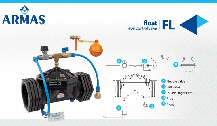
**Armaş "FL"** model float level control valve is the hydraulic control valve designed to control water level in reservoirs and tanks continuously. Main valve is controlled by 2-way modulating type float pilot valve or manually. Main valve mounted on upstream of a reservoir or tank is closed as fully sealed without causing surge when water level reaches to maximum level. Valve opening/closing speed may be adjusted. It may be used in the system by mounting in horizontal or vertical orientations.
